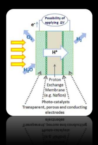
The photo-electrochemical water splitting, or "artificial photosynthesis", is the light-driven splitting of water into H<sub>2</sub> and O<sub>2</sub>
