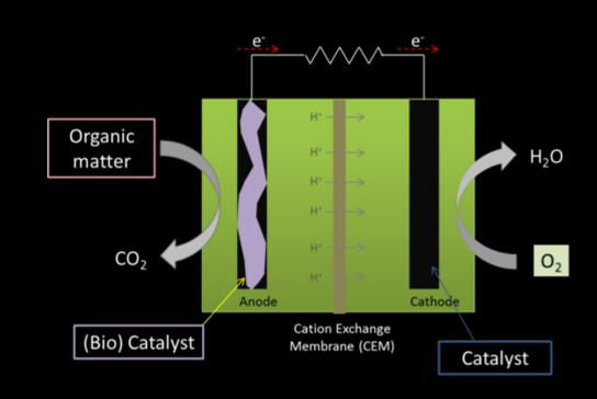
Microbial fuel cells can directly harvest chemical energy from environmental and waste waters.
